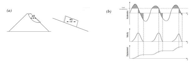
Figure 1. Newmark's Sliding block model: (a) actual slope and sliding block representation of slope subjected to earthquake loading, (b) double integration of acceleration- time history to compute permanent displacement (adopted from Duncan et al. [23])
