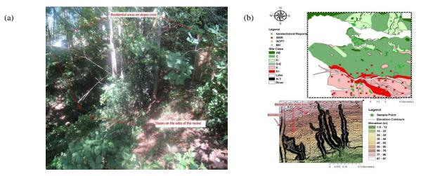
Figure 2. Greater Vancouver region and selected quadrangle in this study: (a) Sample point from field survey in July 21, 2018 (location shown by green star b). (b) Site classes map of Greater Vancouver [26] and available geodata (colored squares; SWR: Surface Shear Wave Refraction, BH: Borehole shear wave velocity logs, SCPT: Seismic Cone Penetrometer).
