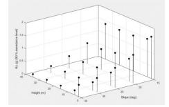
Figure 5. Mean Ky (50% of exceedance) for different slope and height values
